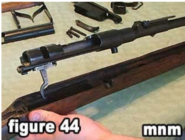
44) Return the barrel and receiver to the stock .
