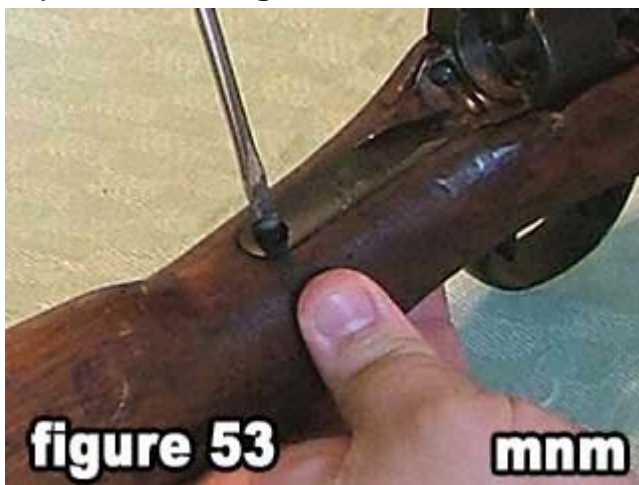
53) Tighten the tang screw.
