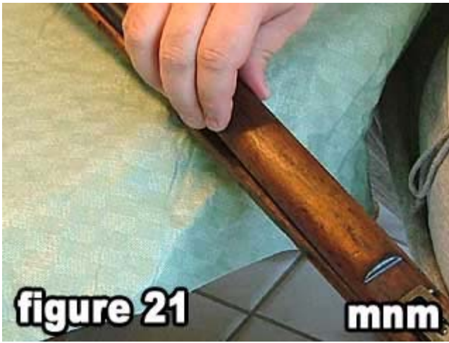
21) Lift the rear sight tang and slide the handguard forward.
