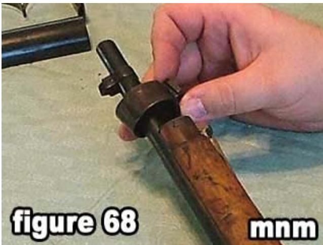
68) Slide the bayonet band over the front sight .
