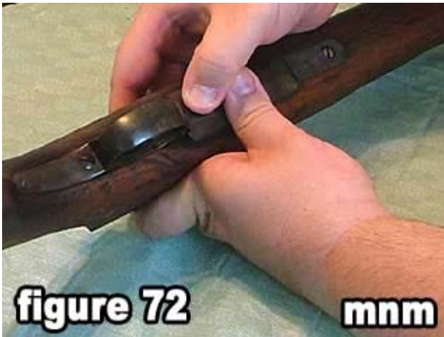
72) Push down on the floor plate until it locks in place.
