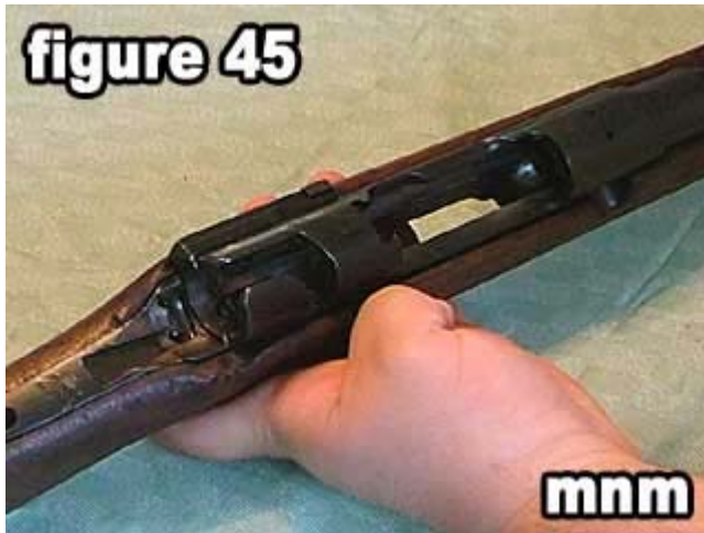
45) Figure 45 shows the receiver properly sitting on top of the upper tang .
