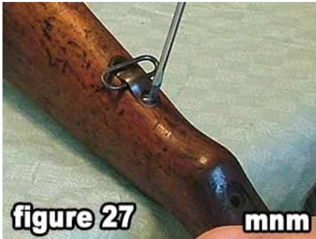
27) Loosen the front swivel screw .
