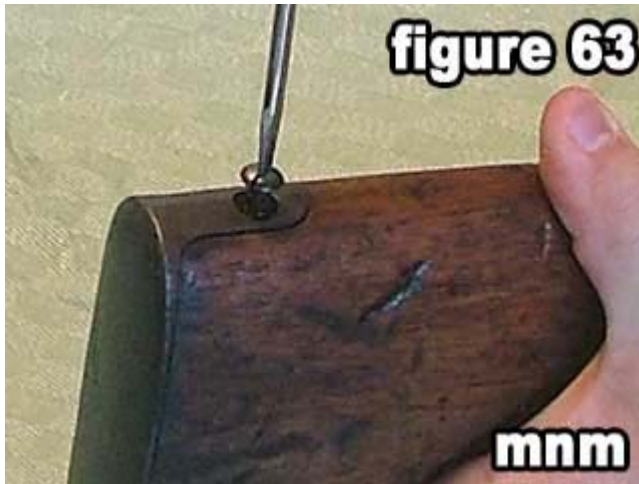
63) Tighten the upper butt plate screw .
