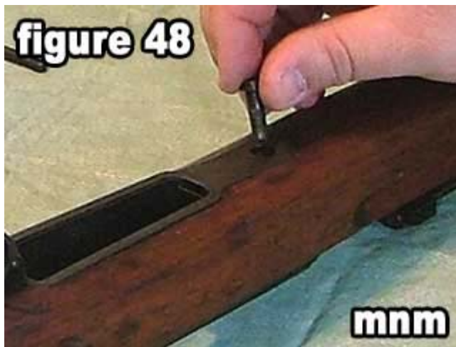
48) Insert the front guard screw.
