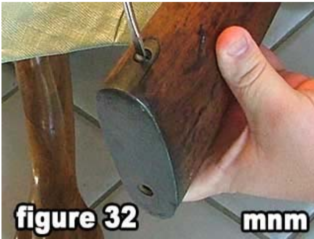
32) Unscrew the upper butt plate screw.
