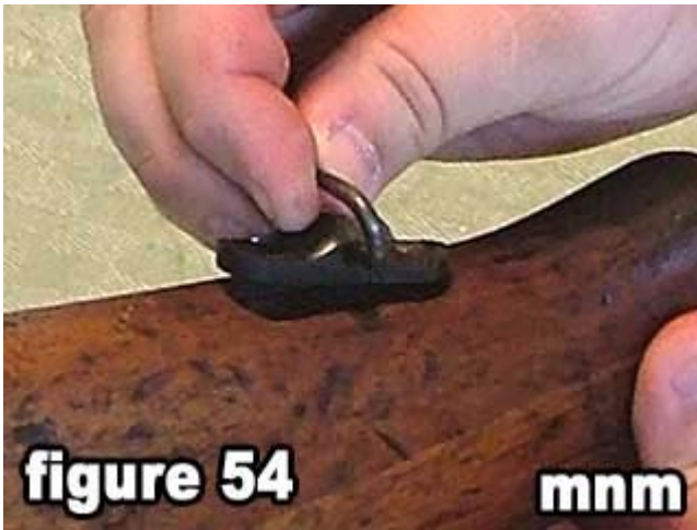
54) Reinstall the rear sling swivel.
