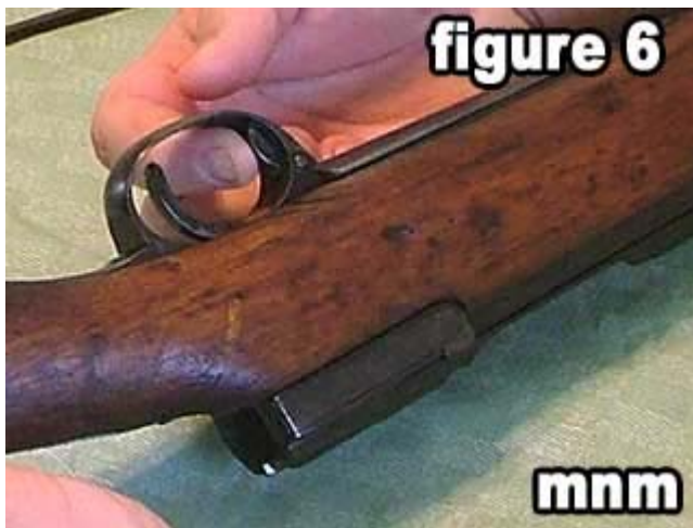
6) Depress the floor plate catch located at the front inside of the trigger guard as shown in figure 6 .
