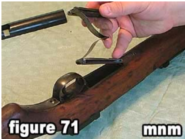
71) Reinsert the floor plate and follower into the magazine well .
