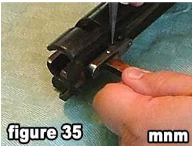
35) Figure 35 shows the sear pin .
