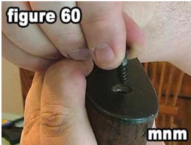
60) Reinstall the lower butt plate screw.
