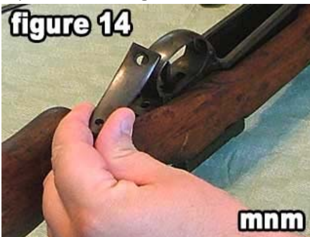
14) Remove the lower tang and set aside.
