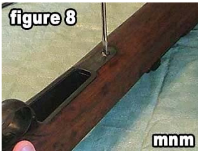
8) Loosen the front guard screw .
