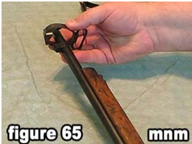
65) Slide the lower band over the front sight .
