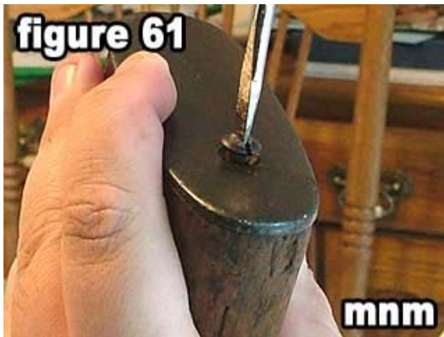
61) Tighten the lower butt plate screw.
