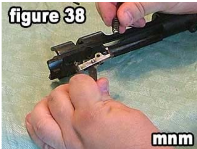
38) Remove the sear spring and set both the trigger and sear spring aside. You have completed the rifle disassembly.
