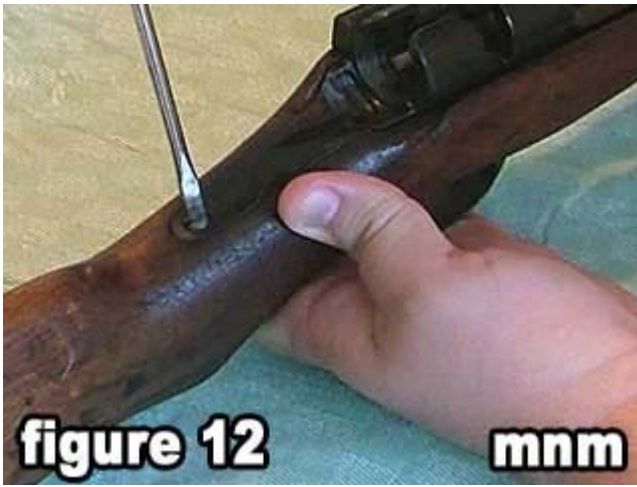
12) Loosen the tang screw .
