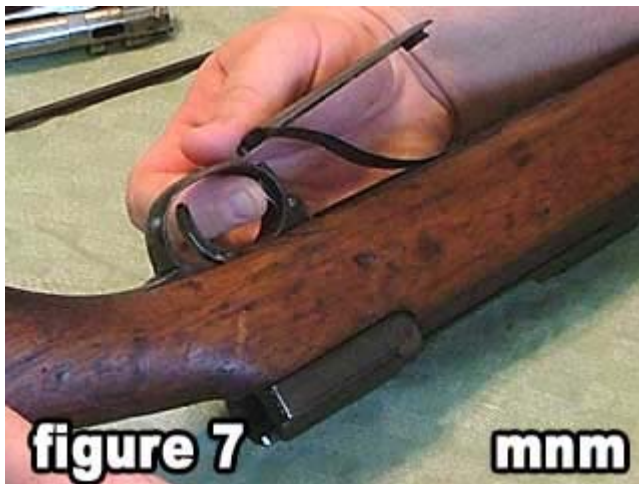
7) Remove the floor plate, follower, and follower spring and set the assembly aside.
