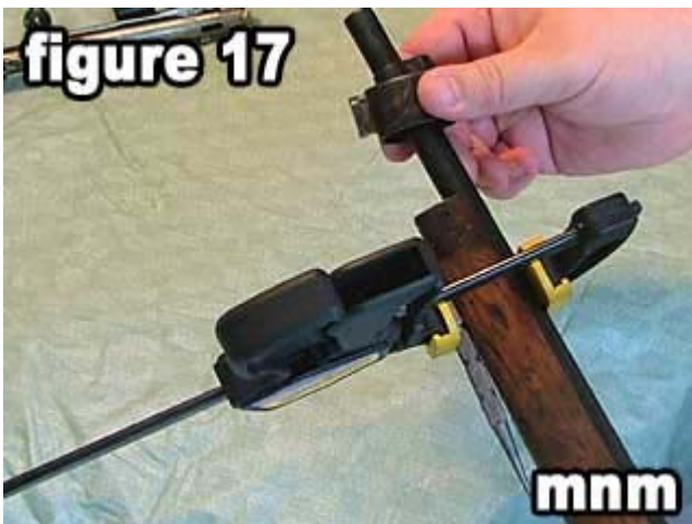
17) Figure 17 shows the removing of the bayonet stud
