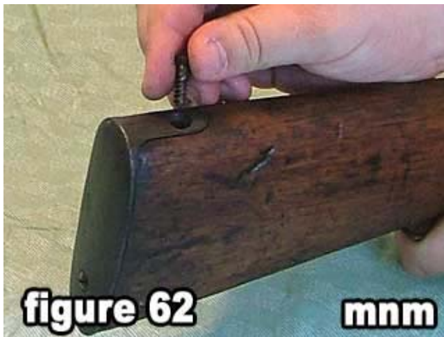
62) Reinstall the upper butt plate screw.
