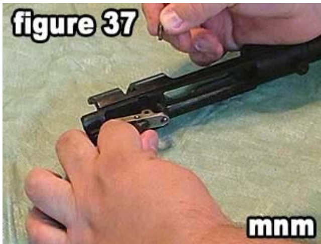
37) Remove the sear pin and set aside.
