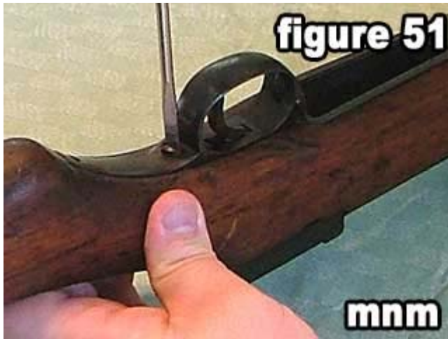
51) Tighten the rear guard screw.
