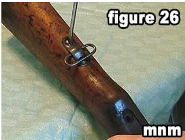
26) Loosen the rear swivel screw and remove.
