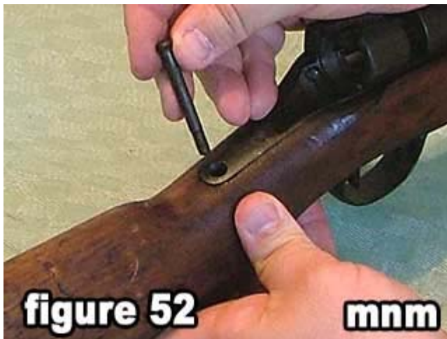
52) Install the tang screw.
