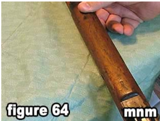
64) Lift the rear sight and slide the hand guard into place.
