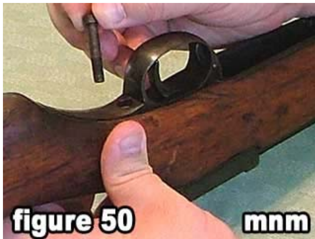
50) Install the rear guard screw.
