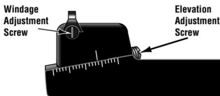
Some T/C in-line muzzleloaders are equipped with a standard rifle rear sight (**Diagram "B" Below**) which is adjustable for elevation by moving the elevation "blade" up or down to change the point of impact. To do this, turn the Elevation adjustment Screw clockwise (as viewed from the receiver end) to lower the point of impact, and counter-clockwise, to raise the point of impact.
