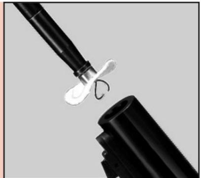
After removing all the fouling, follow up with a few dry patches to thoroughly dry the bore. If the gun is to be stored for any length of time, follow the dry patches up with a good protectant lubricant like T/C's All Natural Lube Bore Butter.
