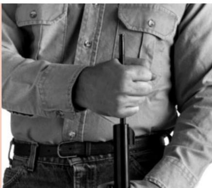
After the projectile is seated tightly against the charge, mark your ramrod to indicate the correct loaded depth of the powder plus the projectile (as shown below)
