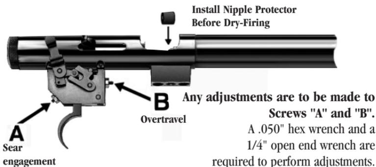
The trigger of the in-line muzzleloader is factory set for optimal weight of pull, sear engagement and overtravel. If further adjustment is required, the in-line muzzleloader is equipped with two trigger adjustment screws that can be adjusted by the shooter. If the shooter is not able to make the appropriate adjustments the adjustments should be made by a qualified gunsmith.
