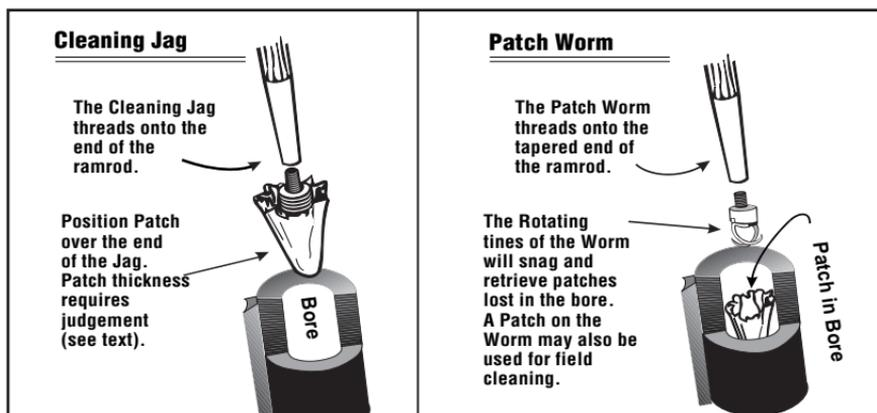
Thompson/Center does not package the worm with each firearm. This is an optional tool and must be purchased separately (one size fits all calibers - see current catalog). The worm is an extremely important muzzleloading tool and every shooter should carry one in his implement bag. While its prime purpose is to retrieve "lost patches", it can also be used for field cleaning. To do so you simply catch the cleaning patch on the tines of the worm and push it into the bore in the conventional manner.
