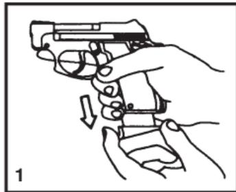
**2. TO LOAD THE GUN.** Hold the magazine with one of your hands and with the other one insert the cartridges one at a time, pressing them down and to the rear. Insert the **MAGAZINE** into the pistol until it is held by the **MAGAZINE CATCH**.
