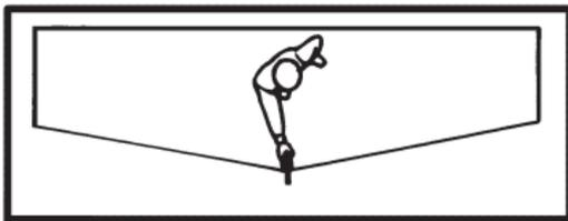
25. If there is any reason to suspect that a bullet is obstructing the barrel, immediately unload the firearm and look through the bore. It is not sufficient to merely look in the chamber.
