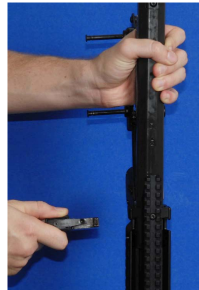
Figure 36: While grasping the carrier and receiver, pull the charging handle straight out to remove it
