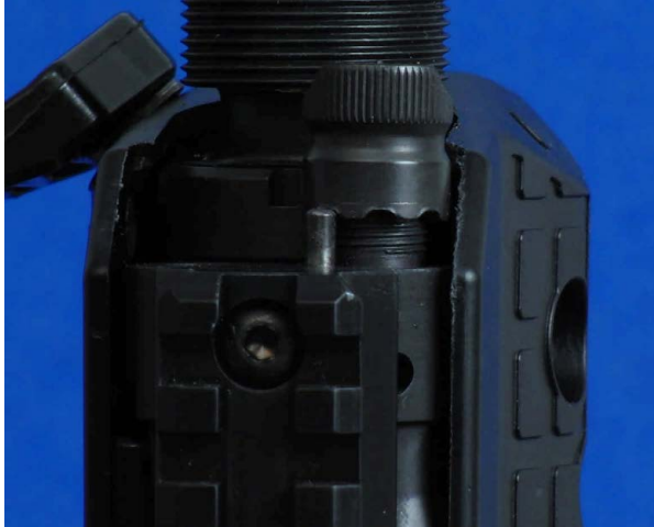
Figure 29: Gas Restrictor Cap set for suppressor use.
