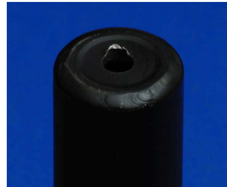
Figure 2: Baffle Strike caused by Subsonic Ammo
