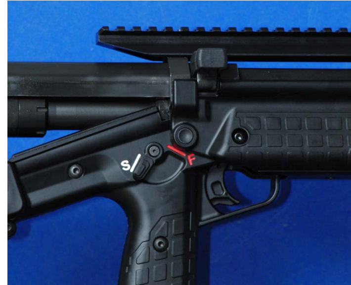
Figure 35: Pull the charging handle back until it aligns with the slot in the handguard to remove it
