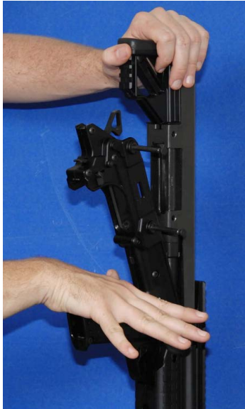
Figure 33: After the pins are pulled out, slap the back of the pistol grip to open the assembly
