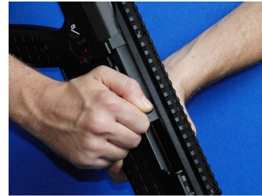
Figure 7: DO NOT RIDE THE CHARGING HANDLE! Release it at its rear most point.
