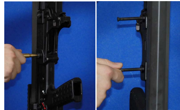
Figures 31 & 32: Use the nose of a bullet to push out the pin.: Be sure to pull out the assembly pins out as far as they will go
