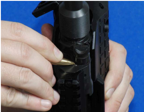
Figure 49: Use the nose of a bullet to push the pin in for disassembly
