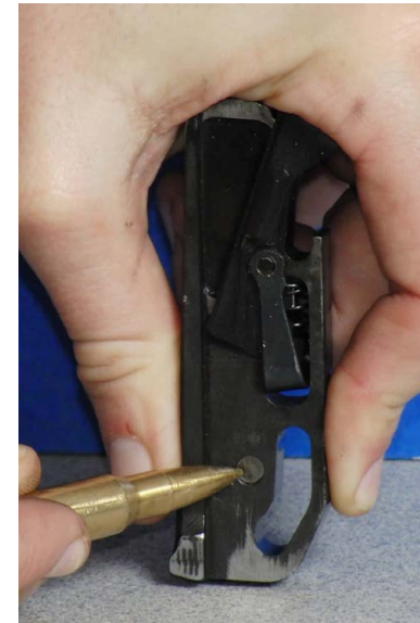
Figure 44: Use the nose of a bullet to push out the firing pin retaining pin
